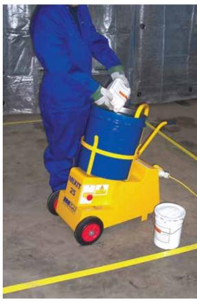
Developed to mix promptly and effectively, quantities of a wide range of materials. The mixer is driven by a sealed motor and gearbox providing many years of trouble-free operation. An optional perforated paddle is available to increase agitation by forcing material through its perforations. The machine is both robust and portable, offering the user high output and single handed operation.
